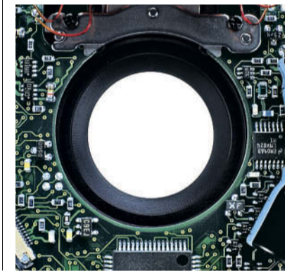
the middle. The light-weight, high-speed blades guarantee precise exposure speed at 1/800 sec
