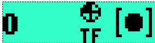
3. Recompose your image, and press the shutter release. The H4D will make a beep sound to indicate a True Focus correction. The AF drive applies the correction, after the mirror has been raised to the UP position, NOT as the camera is rotated.
