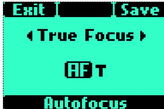
**NB** - In this mode, operation of the AF drive by half pressing the shutter is automatically disabled. All Auto Focus commands are made by the True Focus button.
